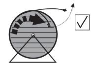
Reeling and unreeling should be done properly in accordance with bending radius suitable for the given cable type and size and its speed should not exceed 60 m/min.
